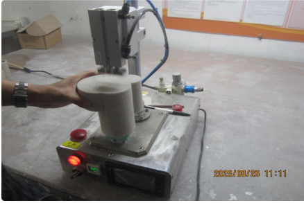
air tightness test
